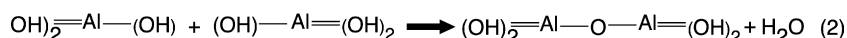
Fig. 2. Reaction set for typical aluminum alkoxides. (1) Hydrolysis is a results of an alcoholysis of the alkoxide (OR) and hydroxy group forming ligand. (2) Condensation is a result of a combination of hydrated ligands coming to form oxygen to metal to oxygen linkages, resulting in water, as a by-product.
